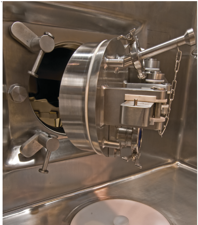
Discharge hatch with sampling port including high containment product offload and heel recovery gloveboxes designed and integrated by PSL
