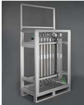
ContiplantPILOT reactor in a vertical arrangement
