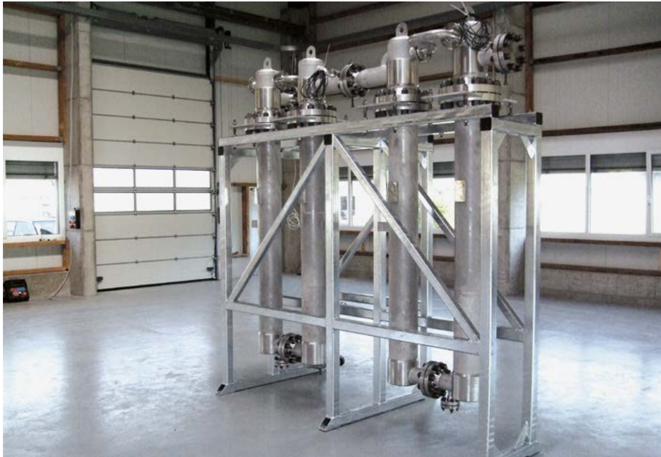
Reaction system scaled up to 4000 kg h -1
