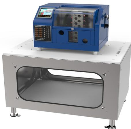
The Coflore® ACR is an agitated cell reactor with a working volume between 30 and 90ml. It is suitable for homogeneous and multiphase mixtures. The ACR reactor block is mounted onto an agitating platform. It has 10 reaction stages and features borosilicate glass viewing windows, side and front entry port which enables multipoint temperature measurement or process connections.
