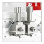
As a dual channel reagent delivery system the **Binary Pump Module** offers users the flexibility to build customised *multi-channel* and *multi-reactor* flow chemistry systems that are able to perform multi-step reaction sequences.
